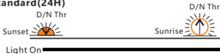
For controllers with "Standard" function(Smart series), if "Time1" is set to "24H" or "7.0H" and sent to the controller successfully, the controller' s load will always open.
