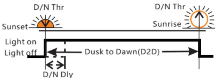
If "Time1" is set to "D2D" ,the controller works in dusk to dawn mode.
